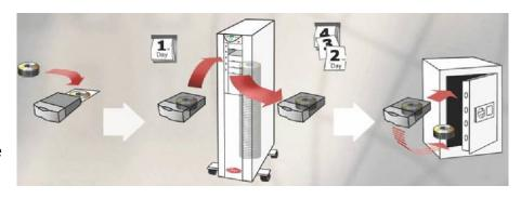
Each SmartPack™ contains a worldwide unique serial number & bar code stored on label and on smart memory chip, so that the storage management software can track the SmartPack™. Unlimited virtual capacity is offered through the efficient handling of the libraries off-line media storage capacity.
