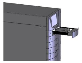
**CAUTION:** Even if the bare BD media are protected by a special hard coating, you must not import media with polluted ore scratched surface into the library! Avoid to touch the read/write area of the media with your fingers! Place exposed media immediately into a well suited case or cartridge!
