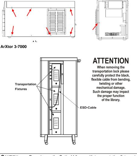
**CAUTION:** Powering on the Optical Library with transportation fixtures inside can damage the robotics. Do not operate the Optical Library while covers are removed. Ambient light will interfere with Optical Library operation, and moving parts increase risk of personal injury.
